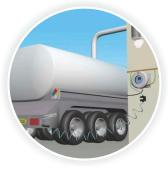
Earthing of road tanker is critical to ensuring static charges do not accumulate on the container (barrel).
